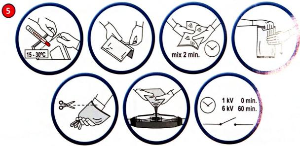
1.13 For joints up to 1000v, joint can be filled under load conditions. The joint should be left for 2 hours before back-filling to allow resin curing process to begin.
