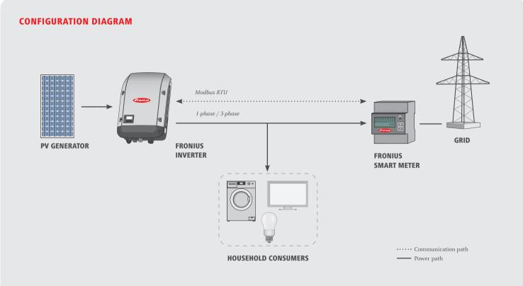
/ The Fronius Smart Meter is compatible with all inverters with an RS485 interface (Modbus RTU). The Fronius Smart Meter works in conjunction with the Fronius Datamanager 2.0 for the Fronius IG<sup>1</sup>, Fronius IG Plus and Fronius CL inverters, whereas the Fronius Datamanager Box 2.0 is used with the Fronius Agilo inverter. The Fronius Smart Meter can be retrofitted at any time together with the Fronius Datamanager 2.0 in inverters that have already been installed.
